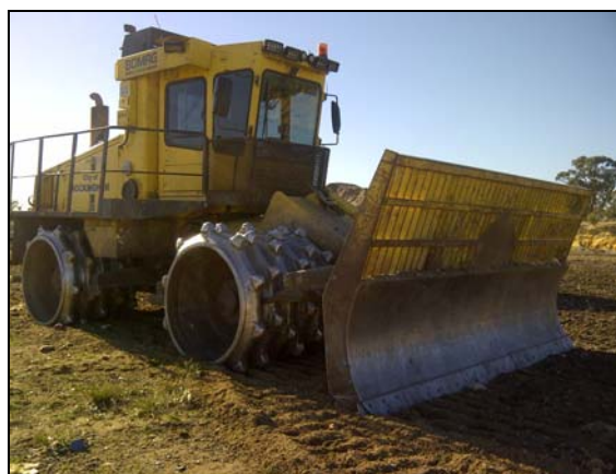
Bomag Waste Compactor
